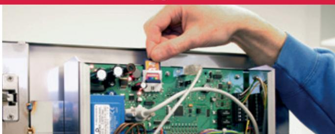
Data logger for optional process documentation and Ethernet connection (IP) for remote request and fault analysis. The data logger records all operating parameters thus ensuring optimum operating and unit reliability.
